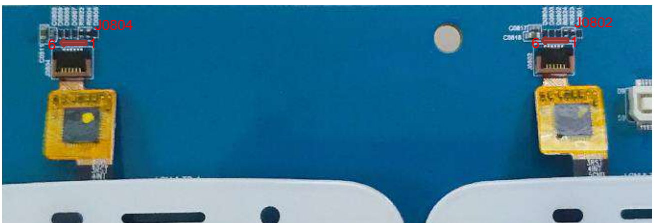
Figure 21: Pin Assignments of Touch Panel Interfaces
