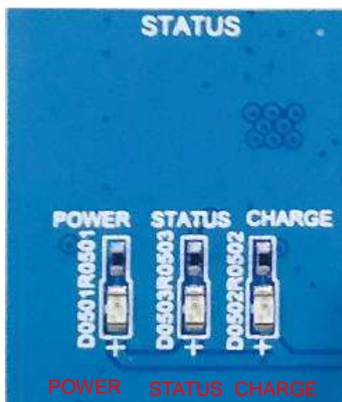
Figure 47: Status Indication LEDs
