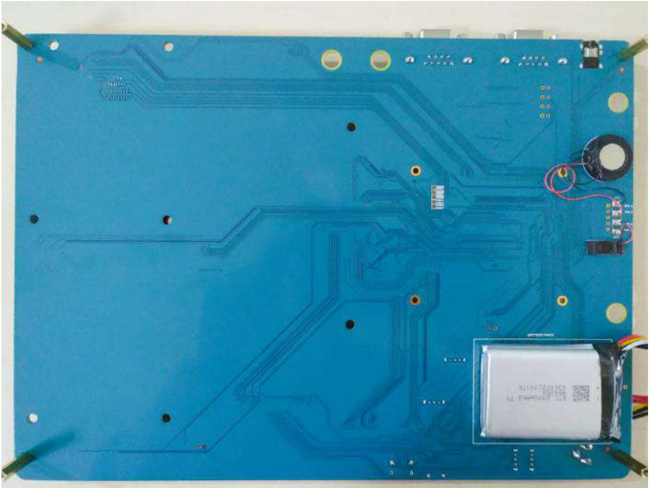
Figure 4: Smart EVB G2 Bottom View
