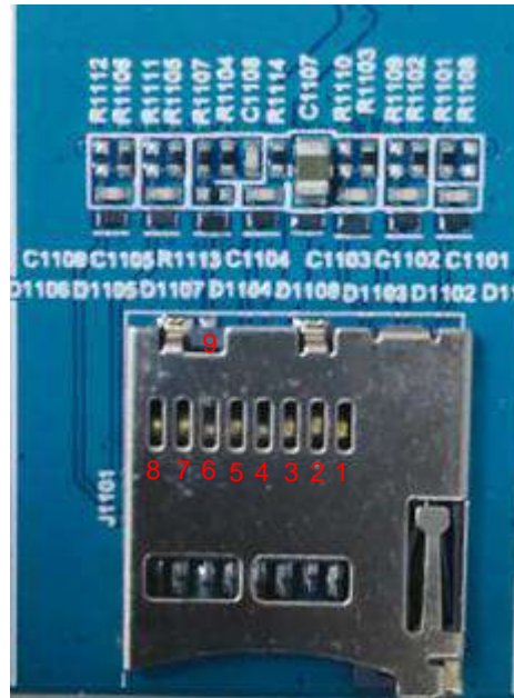
Figure 38: Pin Assignment of SD Card Interface
