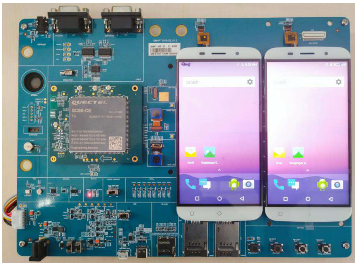
Figure 3: Smart EVB G2 Top View
