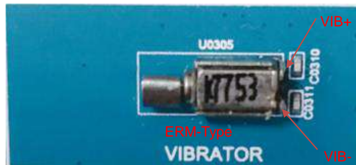
Figure 45: ERM-Type Vibrator
